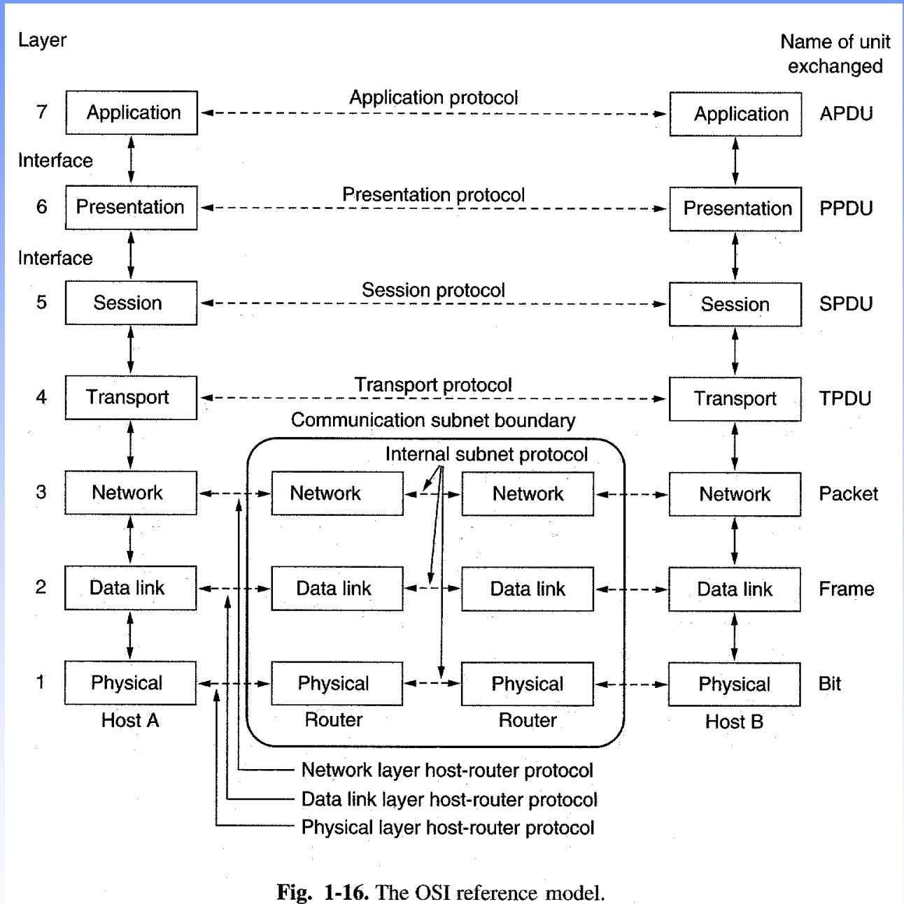
Fig. 1-16. The OSI reference model.
